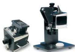
**Reflectance attachment with spectralon integrating sphere**
