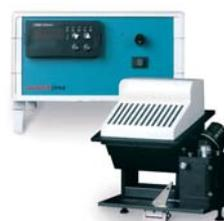
**Peltier-thermostated cell holder with PTC 100 control unit and temperature sensor**
