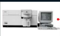
2000 AAS ZEE nit, the first transverse-heated Zeeman graphite furnace AAS instrument with variable magnetic field and 3field mode
