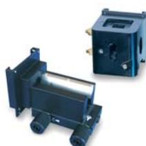
**Thermostated cell holder for 1 cm (or 5 cm) cells (optionally with stirrer)**
