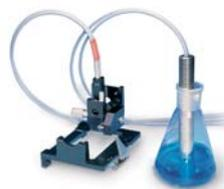
**Fiber coupling with transmission immersion probes and HELMA fiber adapter**
