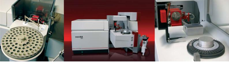
Sample chamber with MPE and graphite furnace Automatic feeding SSA 600
