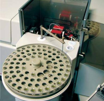
▲ Sample chamber with MPE and graphite furnace
